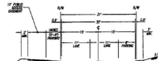
E1 SELVA ROAD EXTENSION PUBLIC STREET SECTION PARKING ONE SIDE N.T.S.
