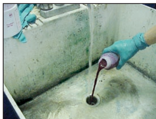
Figure 63: Dye Testing Plumbing (NEIWPCC, 2003)
