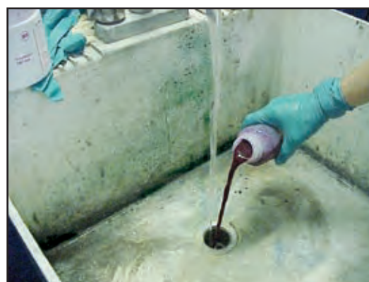
Figure 63: Dye Testing Plumbing (NEIWPCC, 2003)
