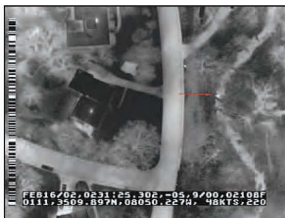
Figure 72: Aerial thermography showing sewage leak
