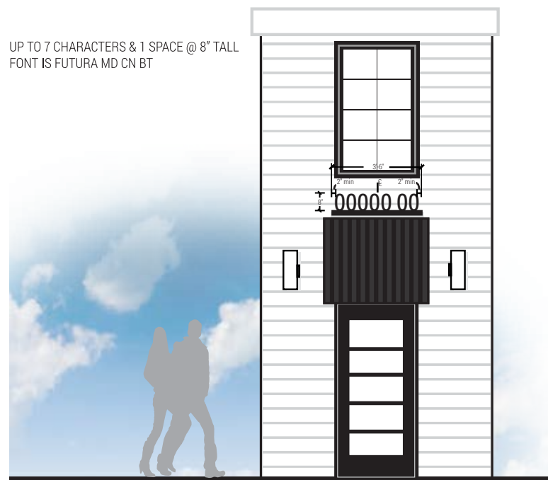
ELEVATION VIEW SCALE: 3/16"=1'-0" SINGLE-DOOR ENTRANCE LAYOUT
