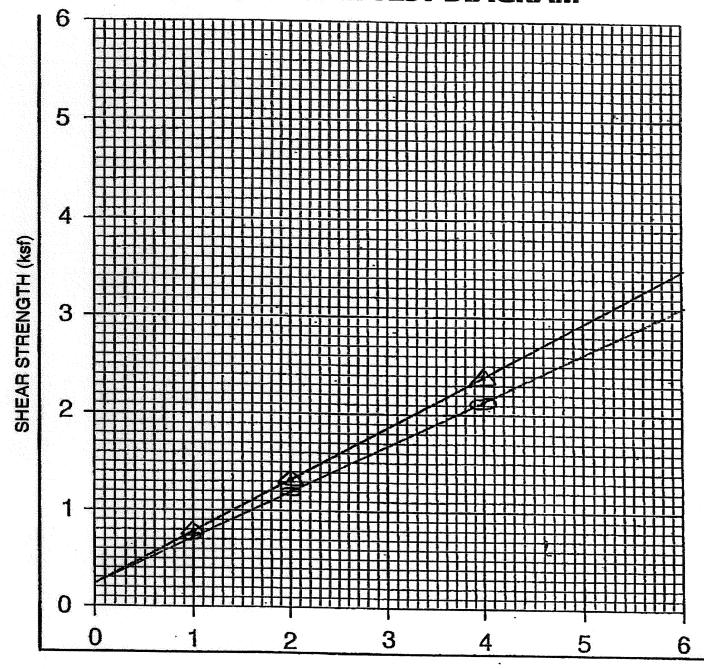
**NORMAL STRESS (ksf)** Boring No. BN-3 Depth 20 and 21 feet Silty Sand w/Gravel and tr. of Clay Soil Description
