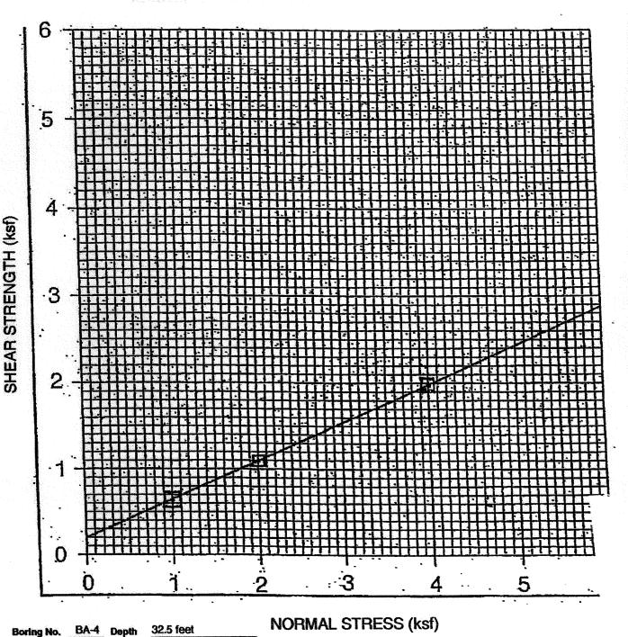
Sandy Silt with Clay **Soil Description** Remolded to 105.5 D.D. Undisturbed/Remolded 19.9% after test Ultimate Reshear Moisture Content, % 0.20 105.7% after test Dry Density, pcf Cohesion (ksf) 99.5% after test 24 **Friction Angle** Saturation, %
